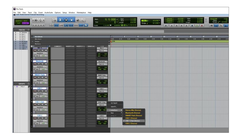
In the I/O section of the channel strip, click on the Input for your 'USB 2' track and change this to 'Interface' > 'USB 2 (Stereo)'.
